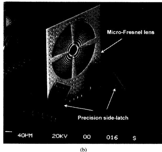
Fig. 2. (a) Schematic diagram of the three-dimensional micro-optics with side latches on both sides. (b) SEM photograph of a three-dimensional micro-Fresnel lens with side latches. The lens diameter is  $280\ \mu\text{m}$ .
