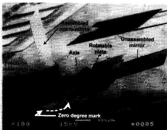
Fig. 3. SEM photograph of a rotatable micro-mirror.
