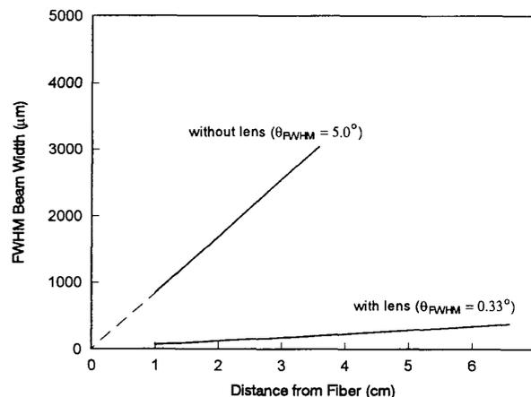
Fig. 4. Collimating performance of the three-dimensional micro-Fresnel lens at  $\lambda = 1.3 \mu\text{m}$ . The intensity FWHM divergence angle of the light emitted from a single-mode fiber is reduced from  $5.0^\circ$  to  $0.33^\circ$  by the lens.
