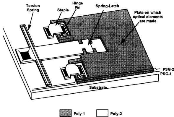
Fig. 1. Schematic structure of the three-dimensional micro-optics fabricated by surface-micromachining. After release etch, the micro-optical plate can be rotated out of the substrate plane and locked by the micro-spring latches.
